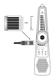
by sound: the "di" sound means connected pair lines, while the "du" sound means short circuit pair lines. All indicator lights of short circuit pairs are on at the same time.
