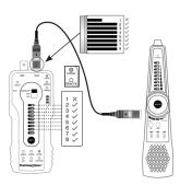
The 1st indicator light is off, indicating that the 1st wire of the port is not connected.
